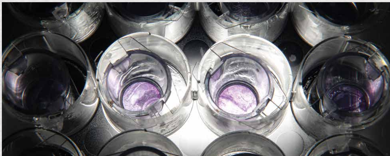
A transwell cell culture system used an in vitro model to evaluate the effects of nutrients and microbes on intestinal mechanisms such as nutrient transport, barrier function, and immune parameters.
